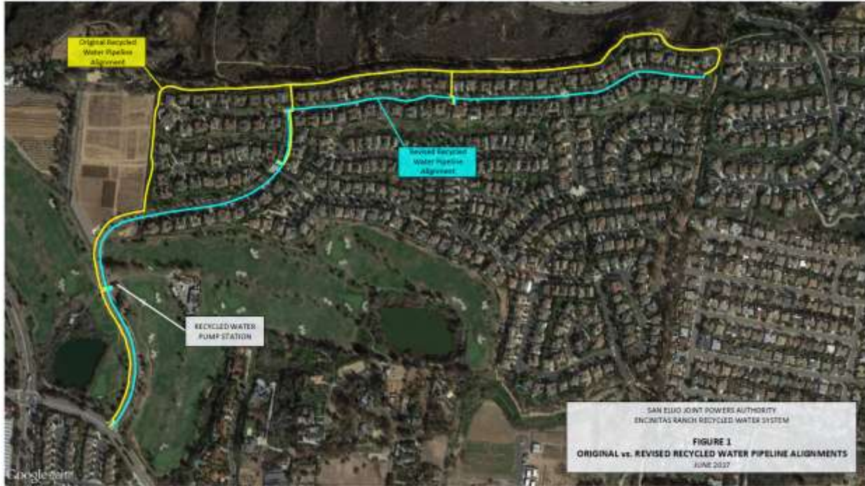
Figure 1 - Proposed pipeline alignment
