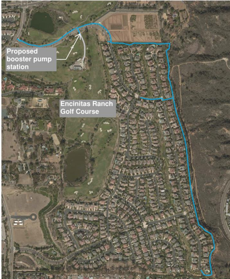
Figure 1 - Proposed pipeline alignment
