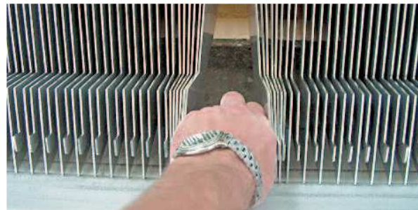
Flexible 0.08" (2 mm) thick lamellae at the bottom of the SSF-HF
